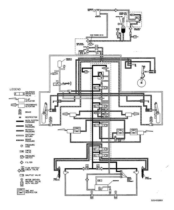
Figure 2-9. Hydraulic System Schematic (Sheet 1 of 2)
